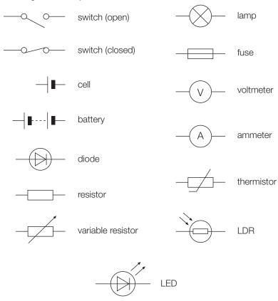
Candidates should understand the use of thermistors in circuits, for example thermostats.
